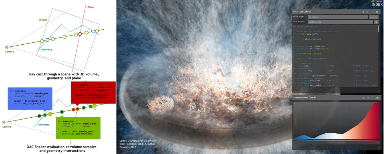
Figure 2. Programming the inner loop of the visualization pipeline. The XAC technology enables scientists to inject CUDA code into the inner loop of the ray-caster/tracer that is then evaluated at each volume sample and at each geometry intersection. The diagram on the left illustrates (top) the volume samples and geometry intersections along a ray cast through a scene and (bottom) that the evaluated XAC shader code determines the color at these positions. The snapshot of NVIDIA IndeX viewer on the right shows a Galactic Winds visualization, the XAC shader code and the color map editor that are both used to create the visualization.
