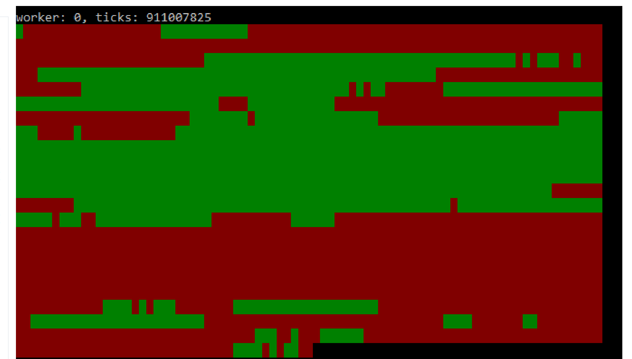
Figure 3: Sample Scheduler Profiling Output, 1 of the many SMs. (Green: Working, Red: Idle)
