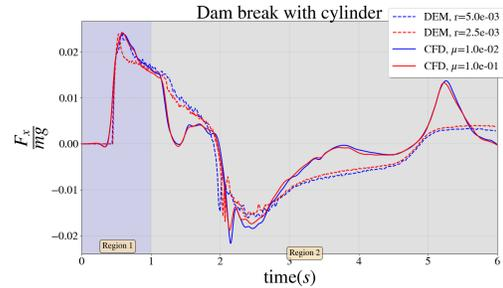
Figure 2: Comparison of the normalized horizontal force experienced by the cylinder in the dam break simulation for different viscosities of the fluid and for different particle diameters of the granular media.
