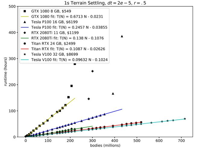
Figure 1: Scaling analysis of a 2-second terrain settling simulation
