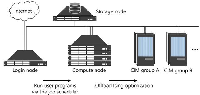
Figure 2: Configuration of LCS.
